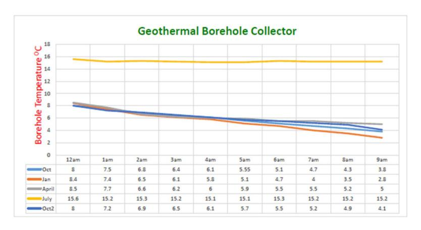
Performance data of borehole collector recording a full year of data in Kellys Toyota from October 2010 to October 2011. Note the high temperature of the boreholes in July – this is due to the passive cooling of the Showroom that is being transferred to the collector.
